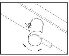
12. Rotate the "CAM" handles on the hold back bars 180° to the open position.
