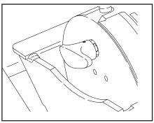
7. Disengage the winch "free-spool" by pulling out on the "T" handle and turning the handle 90°. The handle should remain in the "free-spool" position. Never turn this handle while the wire rope is under load! This allows the wire rope to be pulled directly off the drum to the work.
