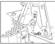
27. Swing the hold back bars in toward the tow sling storage brackets on the side of the boom. Allow the hold back bars to retract as necessary.
