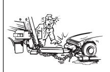
Never attach the chain hooks in such a way as to damage brake lines or other functional parts.
