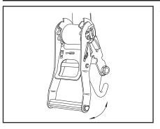
To release the ratchet, simply pull on the locking bar, disengaging the teeth and raise the handle to the "free spool" position.
