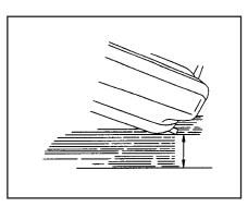
16. Raise the vehicle into the final towing position observing the far end for sufficient ground clearance. It is possible to set the rear of a front lifted vehicle completely onto the ground, causing damage. Take irregular roadsurfaces into consideration. Observe the lift function from the side and away from both vehicles if possible.
