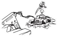
Don't disengage the winch drum clutch while the wire rope is loaded.
