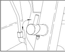
Rotate the "CAM" handles on the hold back bars 180° to the open position.
