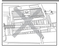
11. With the wire rope tight, slowly wind it in, observing both the work and the drum. Be sure the wire rope strands do not cross wrap or criss-cross on the drum. Observe the path the work must travel for snags or obstructions which could stall the movement and overload the wire rope.
