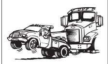
Don't pick-up and tow a vehicle that reduces the weight on the front wheels of the wrecker more than 50 percent.
