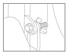
Remove the retaining bolts and wing nuts or pad locks, which ever your unit may have.
