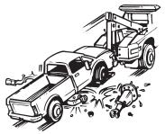
Don't tow a vehicle on its drive wheels unless steps have been taken to protect its transmission and differential. Follow the recommendations of the vehicle manu-facturer. As an alternative, use a towing dolly.
