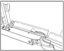
Attach the lower trough and vertical stop into the mounting bracket at the front of the boom with the pin and retaining pin.
