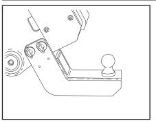
4. Install the desired towball to the towball hitch.
