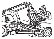
• Be sure the chains and hooks are attached to frame members and not sheet metal.
