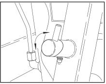
29. Rotate the "CAM" handles on the hold back bars 180° to the closed position.
