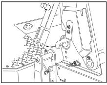
Swing the hold back bars out toward the lower tow sling lugs on the back of the body. Allow the hold back bars to extend as necessary.
