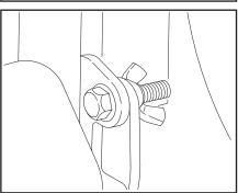
16. Install the retaining bolts and wing nuts or pad locks.
