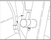
Rotate the "CAM" handles on the hold back bars 180° to the close position. Raise or lower the boom slightly until the cam locks on the tow sling hold bars snap into the closed position.
