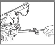
8. Extend the wrecker boom and adjust the wire rope cable(s) to lift the top of the tow sling and tow sling straps.
