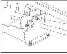
8. Install the retaining bolts and wing nuts or pad locks.
