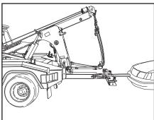
10. Carefully extend and lower the wrecker boom to allow the tow sling head to rotate outward and down away from boom.
