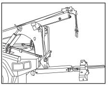
Position the boom head by using the boom up and down control lever and the boom in and out lever.
