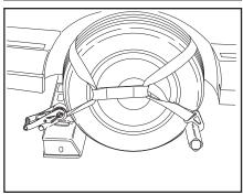
Raise the wheel grid to the towing position. RE-TIGHTEN THE RATCHET PERIODICALLY AS THE TIRE SETTLES IN GRID FROM TOWING.
