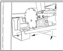
Afterloading the dollies, place the pry bar/jack bar back into the storage bracket by inserting the end of the bar with the ring around it thru the cutout in the front bracket. Allow the other end of the bar to rest on the rear bracket.
