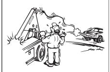
Never completely unwind wire rope from a winch while loaded. Always be sure that a minimum of five (5) wraps of wire rope are on the drum at all times.
