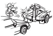
All boom placement functions should be made with the winch wire ropes set in "free spool" to avoid over tensioning or breaking the winch wire ropes.
