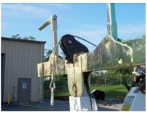
7. Route the winch wire rope/cable over the sheave and install the guide pin in the outer most hole to retain the cable.
