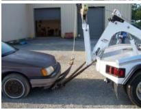
Maneuver the sling under the vehicle to be towed, and far enough under so the vehicle will ride on the rubber belts.
