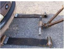
13. Remove the right hand and left hand tow sling straps for the toolbox and lay them out next to the hold back bars on their respective sides.
