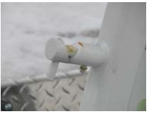
11. Position the lower anchor assembly on the ground behind the truck and turn the "CAM" handles on the back bars 90°.
