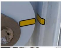
Fold the underlift up until the alignment indicators on the underlift and on the knee boom match up.
