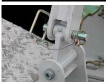
Connect the hold back bars to the tow sling lugs using the pins that you removed earlier.
