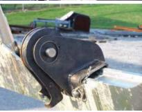
Take the underlift sheave assembly from the toolbox and install it onto the underlift crossbar using the pins provided.
