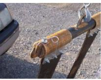
16. Install the upper heads of the strap assemblies onto the ends of the upper anchor assembly securing the heads with the snap pins provided.
