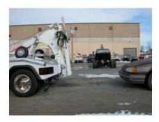
Position the truck within 9 ft. of the casualty vehicle and as close to the direction of the tow as possible.
