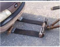
14. Install the lower heads of the strap assemblies onto the ends of the lower anchor crossbar. Be certain that the hook opening faces toward the truck and away from the casualty vehicle. Wrap the straps under the crossbar from front to rear. Secure the heads with the snap pins provided.
