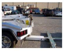
2. Lower the boom and unfold the underlift.
