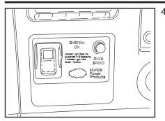
Engage the Power-Take-Off 4. (PTO) or Clutch Pump and the hand controller using the "Control" switch in the switch panel. Most trucks will automatically throttle up when the parking brake is set and the transmission is park or neutral. NEVER TRAVEL WITH THE POWER-TAKE-OFF or CLUTCH PUMP CONTROL **ENGAGED.** This could result in damage to the PTO or Clutch Pump unit and the truck transmission.
