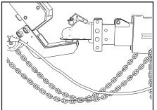
6. Connect the trailer lights and attach safety chains.
