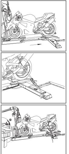
12. After securing the front tire, extend the wheel lift under the rear tire of the motorcycle raising the rear tire of the motorcycle onto the ramp.
