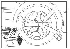
3. Place the hook of the ratchet into one of the holes on the front side of the grid. Again, try to use the hole that is closest to the tire.
