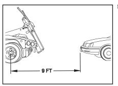
5. Confirm the truck's position in relation to the vehicle to be towed. Nine (9) feet is recommended. Reposition the MPL if necessary. Be sure the towed vehicle is not in gear or park. Keep the brake set.
