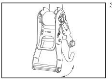
3. To release the ratchet, simply pull on the locking bar, disengaging the teeth and raise the handle to the "free spool" position.
