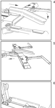
4. Hook the loading ramp onto the wheel grid and engage the rear hooks on the back side of the grid.
