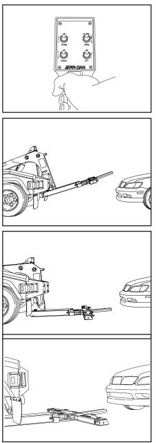
6. Using the hand controller, unfold the underlift using the tilt down function. The underlift level stop assist system will stop the underlift travel at a preset position.
