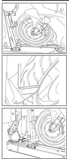
9. Push the motorcycle up the ramp until the front wheel is resting in and against the tire stops in the front brackets.
