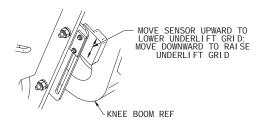
NOTE: A GAP OF .125-.1875 MUST BE MAINTAINED BETWEEN THE SENSOR AND THE BASE BOOM SIDE PLATE. INTERMITTENT OPERATION WILL OCCUR IF THE GAP IS NOT MAINTAINED.
