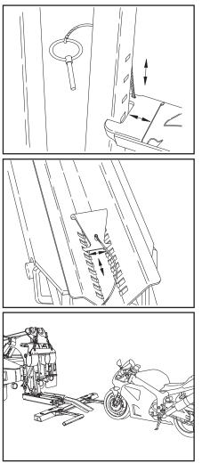
7. Adjust the upper and lower tire stops so that they will contact and restrain the front tire when loaded.
