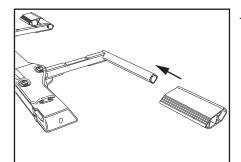
1. Slide the back side of the wheel spacer over the wheel grid arm.
