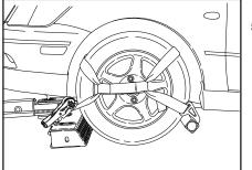
5. Raise the wheel grid to the towing position. **RE-TIGHTEN THE RATCHET PERIODICALLY AS THE TIRE SETTLES IN GRID FROM TOWING.**
