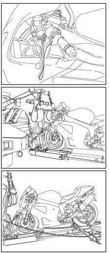
15. Tie the front of the motorcycle to the rear of the wrecker body. Attach the lasso style straps to each of the handle bars.
