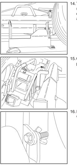
14. The tab on the storage bracket should be placed through the dolly pocket of the dolly wheel assembly.
