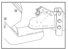
5. Position the ball coupler over the ball and lock into place.
