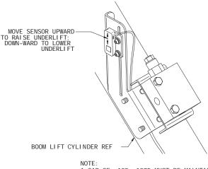
A GAP OF .125-.1875 MUST BE MAINTAINED BETWEEN THE SENSOR AND THE DOUBLER PLATE. INTERMITTENT OPERATION WILL OCCUR IF THE GAP IS NOT MAINTAINED.
