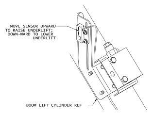
NOTE: A GAP OF .125-.1875 MUST BE MAINTAINED BETWEEN THE SENSOR AND THE DOUBLER PLATE. INTERMITTENT OPERATION WILL OCCUR IF THE GAP IS NOT MAINTAINED.
