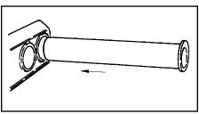
3. Insert the round tube into the desired position in the grid.
