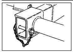
7. Install the retaining pin through the grid and arm weldment and secure with the pin.
