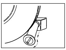
Using the pulling tool, extend the round tube to capture the back of the tire. After extending the tube, make sure that the flanged edge of the tube is turned up to prevent the tire from sliding off the end of the tube.
