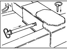
1. Slide the tire lift grid onto the crossbar.
