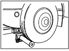
Extend the under lift under the casualty vehicle so that the arm makes contact with the front of the tires. At the same time make sure that you are not going to damage any under body components.
