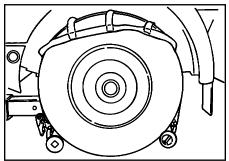
11. Attach the hook end of the tiedown strap to the round tube behind the tire. Pull the strap up and cover the tire and attach the hook on the ratchet end of the strap to the arm in front of the tire.
