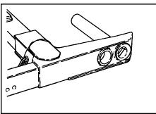
5. Retract the tube inward to the loading position.
